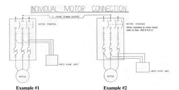
When using the *Example #2* connection for the installation of the Power Factor Correction Bank, the overload sizing for the motor protection would determined by deducting the "Nominal Amperage" rating of the Power Factor Correction Bank from the recommended overload sizing for the motor load.
